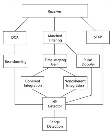
The preceding figure only presents an overview of the array signal processing operations supported by the software rather than predetermined orders of operation. For example, direction of arrival (DOA) estimation, beamforming, and space-time adaptive processing (STAP) often follow operations that improve the signal-to-noise ratio such as matched filtering. You can implement the supported algorithms in the manner best-suited to your application.
